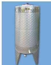
Stainless steel fermentation tank 240l (pressureless) with cooling jacket and feet Ø 820 mm, H 1466 mm Outlet for clear wort ¾" female thread Total outlet ¾" female thread Item No.: FD-082-S Var 0023
