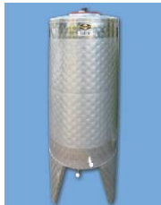
Stainless steel fermentation tank 240l (pressureless) with cooling jacket and feet Ø 550 mm, H 1524 mm Outlet for clear wort ¾" female thread Total outlet ¾" female thread Item No.: FD-055-S Var 0008
